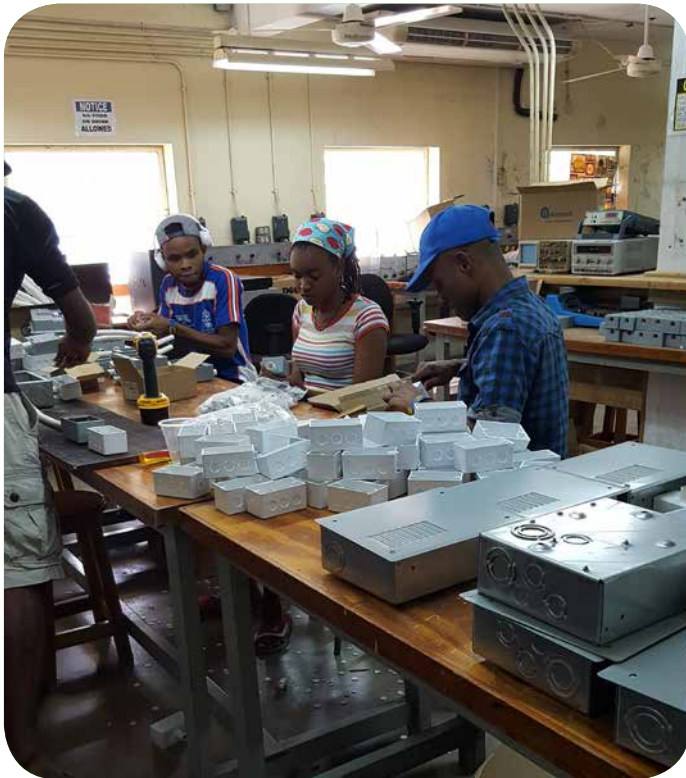
School of Engineering students working diligently with materials to construct 400 electrical power supply Ready Boards. From left are Wardlan Borah, Sheveena Haye and Jeremy Mcray.
